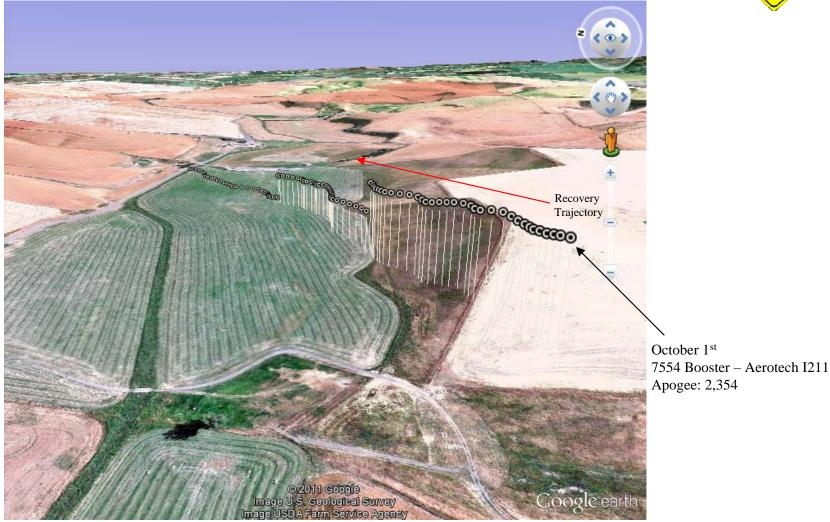
The actual flight exceeded site boundaries by close to 500 feet landing east of the launch site and across the gravel road.
