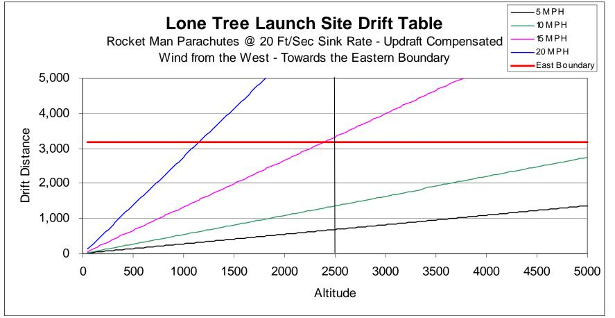
Based on the Updated BMR Drift Chart, now compensated for the updrafts, this flight would not have been allowed due to the launch site boundary safety code constraint.
